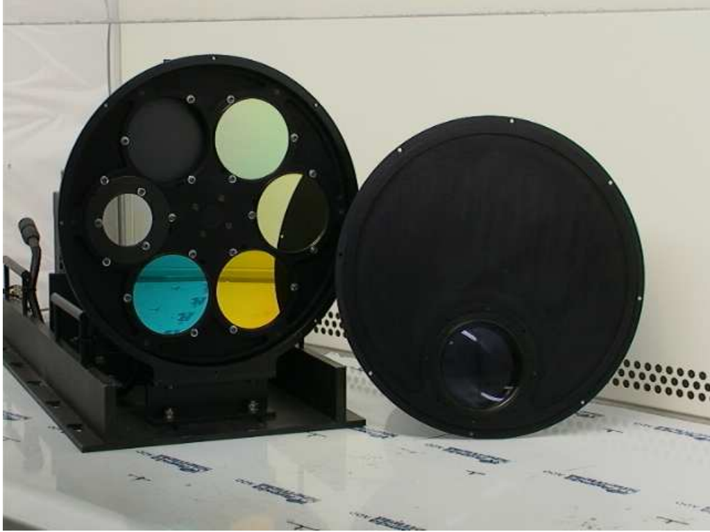
Figure 3.8: The six-position filter wheel with cover removed exposing the filter compartment. Starting at filter position zero (approximately five o'clock in the photo) filters for: O(^1S) 5577 Å, O(^1D) 6300 Å, 6230 Å (background), white light (empty), 5324 Å (a smaller filter in an adaptor ring intended for LIDAR studies), and finally in position five, the N_2^+ 1Neg. 4278 Å auroral filter. To the right the cover with the back end of the front lens is seen. A stepping motor attached to the rear top side of the filter wheel enclosure (not shown) actuates the filter wheel by a small cog-wheel driving cogs in the inner perimeter of the filter wheel. An angular encoder is attached to the filter wheel axis on the rear side of the enclosure (not shown).
