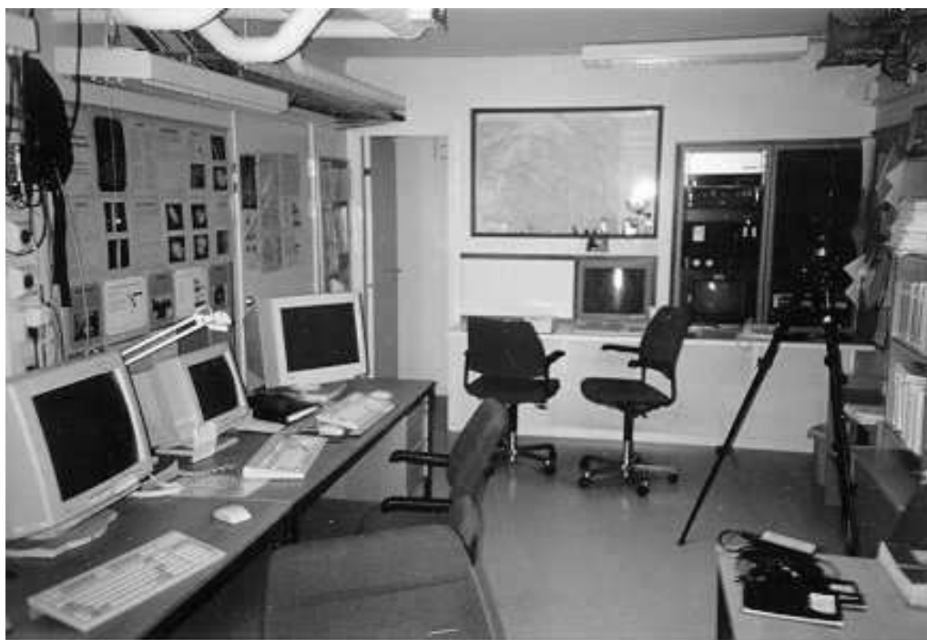
Figure 2.6: The ALIS control centre at the optical laboratory as it looked around 1993. To the left are workstations and the station computer for the Kiruna station. The station overview map and console for the HP-755 workstation are seen in the center-right part of the photo. The two racks to the right contains monitors for the low-light TV-cameras, video recorders and timing systems.
