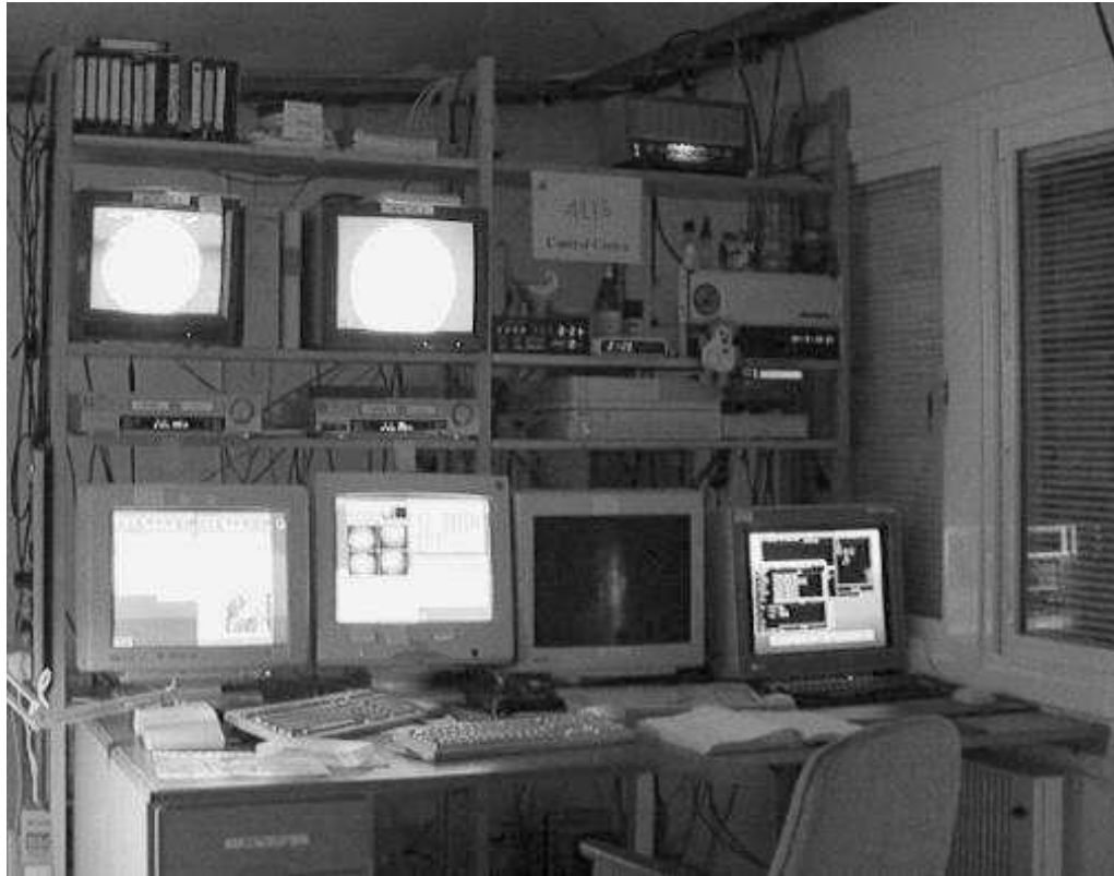
Figure 2.8: The ALIS operations centre that was established at Knutstorp (close to the EISCAT-site in Kiruna) in 1999. Two low-light TV-cameras (one with all-sky, and one with \approx 40^\circ field-of-view) are used to give the operator a real-time display of the sky. These images are displayed on the monitors in the upper left part of the photograph. Below are two video tape recorders. The six ALIS stations are monitored and controlled from the computer terminals below, and some quick-look images from ALIS are seen on the screens.
