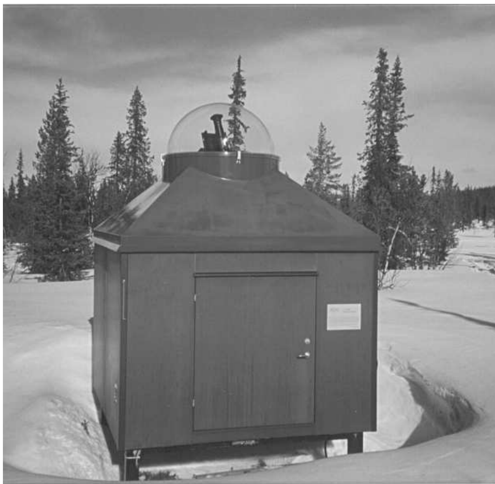
Figure A.3: The GLIP in Tjautjas (4) showing how snow is prevented from building up around the station.
