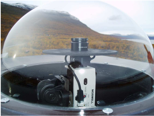
Fig. 4. A photo of the all-sky dome and the CCD unit at Abisko Turiststation. The dome is installed over the building's roof room where the computer and ventilation is installed. The black part at the top is the fish-eye lens, and the white box underneath is the CCD camera.
