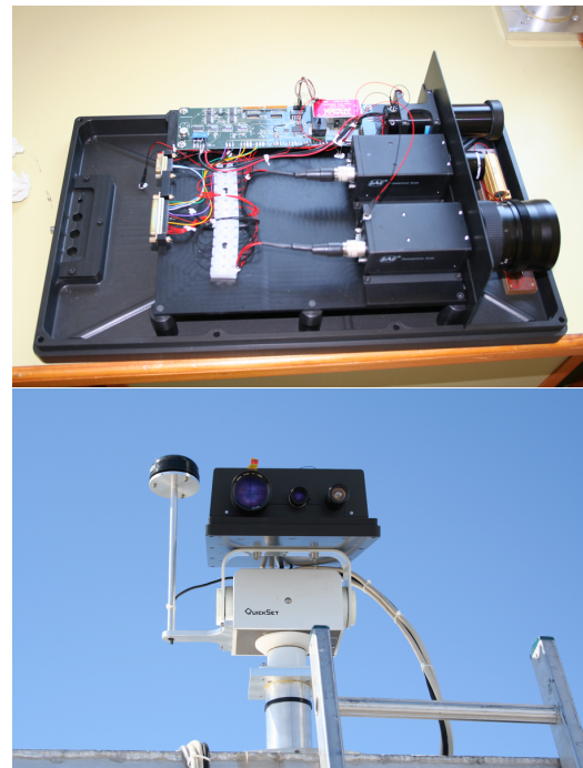
Fig. 2. The Pic du Midi camera system. Upper picture: The mounting of the two JAI cameras. Lower picture: View of the setup, cameras mounted on the pan-tilt unit.
