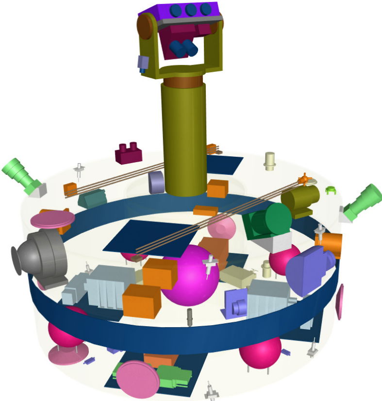
Figure C.17: ESCAPE satellite subsystems view.
