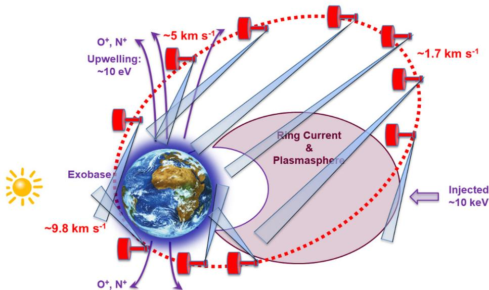
Fig. 2.2. Example of remote-sensing instruments pointing strategy, along the various portions of the ESCAPE orbit. The two degrees of freedom pointable despun platform allows a large flexibility in acquiring imaging data.
