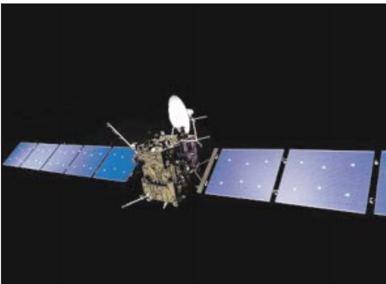
Artist's impression of Rosetta. The sensors of the IRF-Uppsala LAP instrument are mounted on the two long booms that extend from the spacecraft body (ESA).
