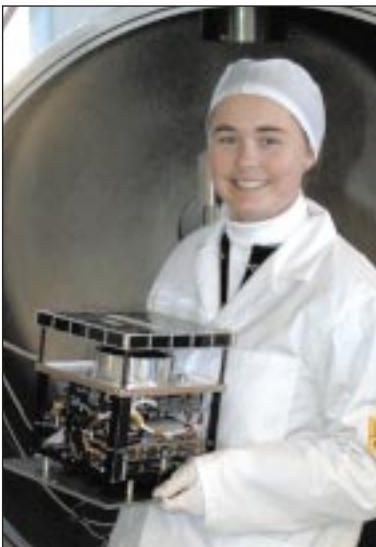
IRF's nanosatellite Munin, due to be launched in late 2000, weighs only 6 kg.
