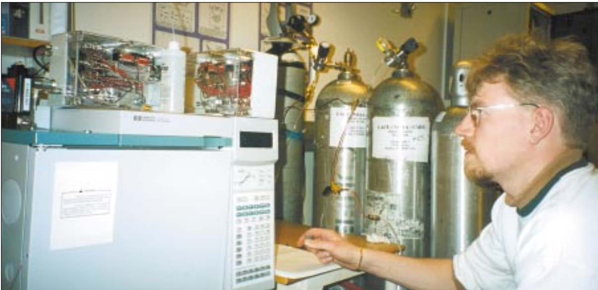
PhD student Johan Arvelius oversees the gas chromatograph read-out from the DESCARTES instrument. Photo: Hans Nilsson.
