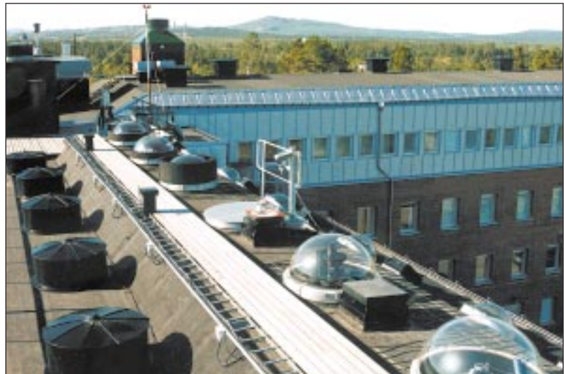
Instruments on the roof of the Optical Laboratory at the Kiruna Division include all-sky cameras and spectrometers. Photo: Torbjörn Lövgren.
